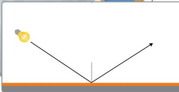
Gloss is measured by directing a constant intensity light beam, at a fixed angle, on to the test surface and then monitoring the amount of reflected light from the same angle. This specular reflectance is measured using a glossmeter.
