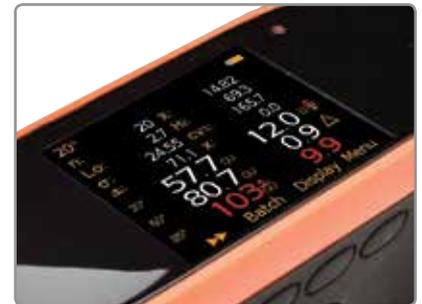
In order to avoid subjectivity between inspectors, the Elcometer 480 can automatically generate and store the nominal (target), highest & lowest acceptable gloss values (Limits) from the Master Standard.
