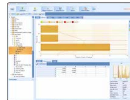
Combine multiple inspection parameters (Material thickness and profile) into bespoke reports.
